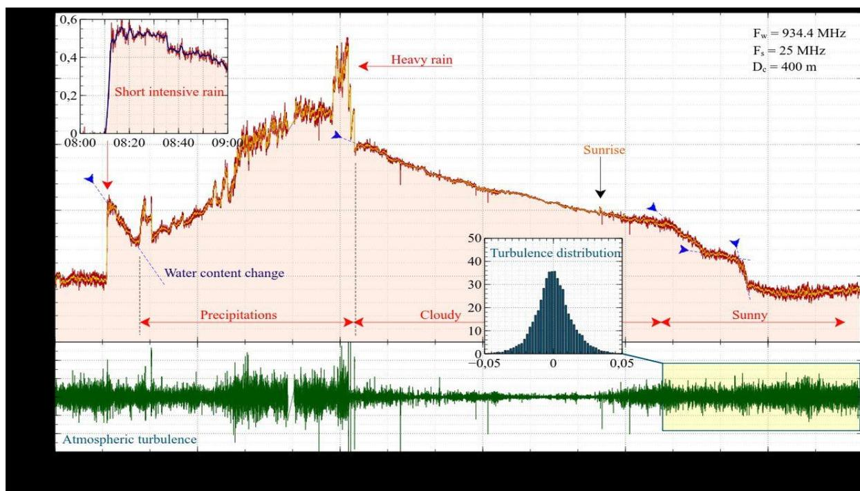
Fig. 11. Signal response to the hydrometeors occurrence within 50 m layer over the ground
