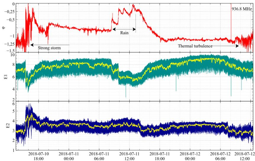
Fig. 10. Phase displacement and energy values measured during the cold front passage
