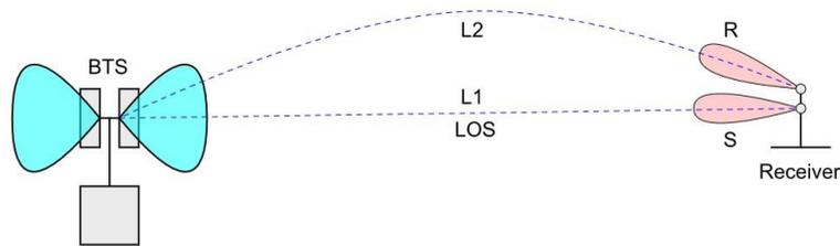
Fig. 7. Configuration and antennas alignment and their Fresnel patterns
