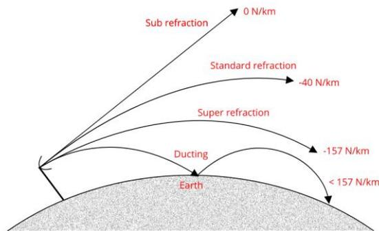
Fig 3. Examples of electromagnetic waves propagation in the atmosphere
