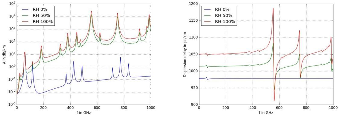
Fig. 4. Model MGM93 - attenuation and the delay of the signal for various values of relative humidity
