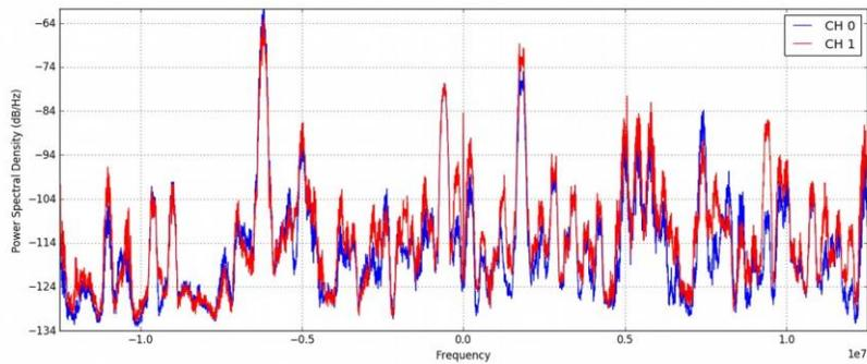
Fig. 9. Spectrum of the signals calculated from ID components, mean frequency corresponds to 930 MHz
