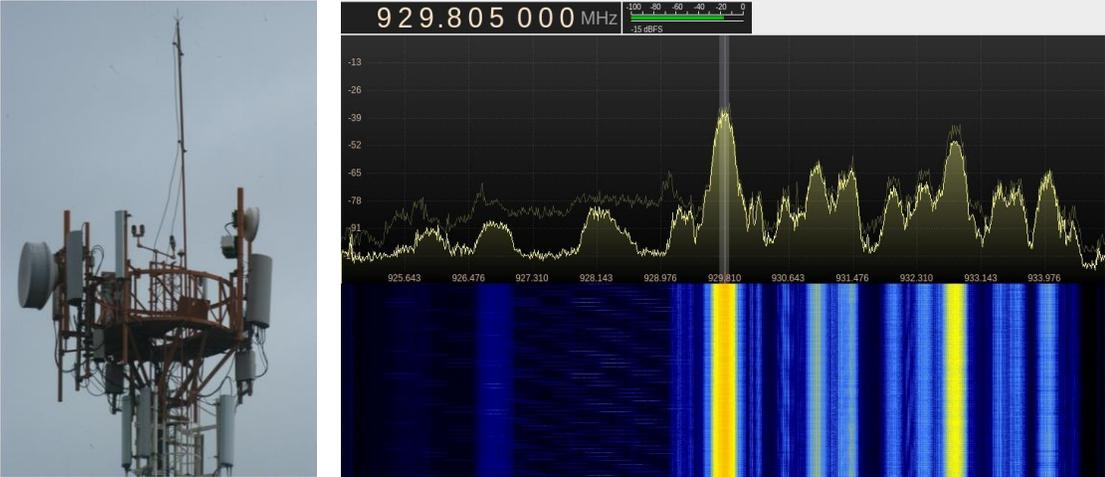
Fig. 6. BTS and power spectrum of a part of the band of mobile G2 network
