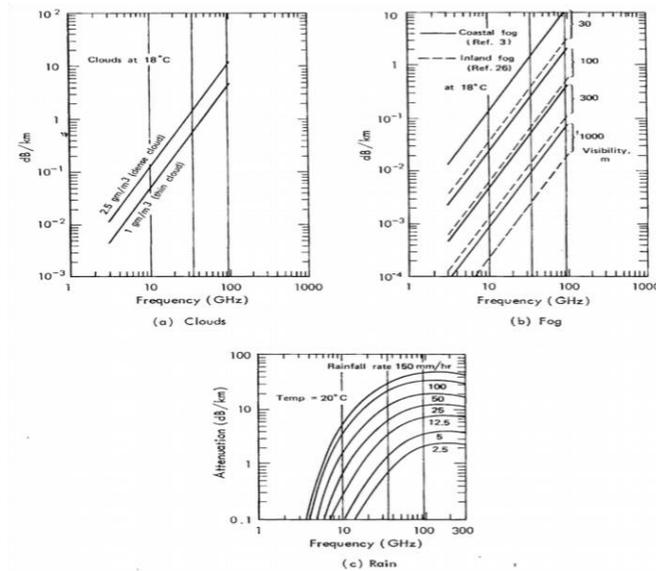
Fig. 5. Results of the experimental measurements of signal attenuation due to hydrometeors [8]
