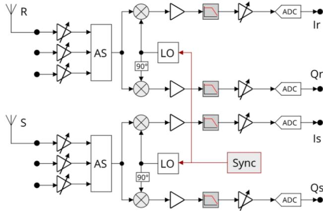
Fig. 8. Block scheme of the receiver
