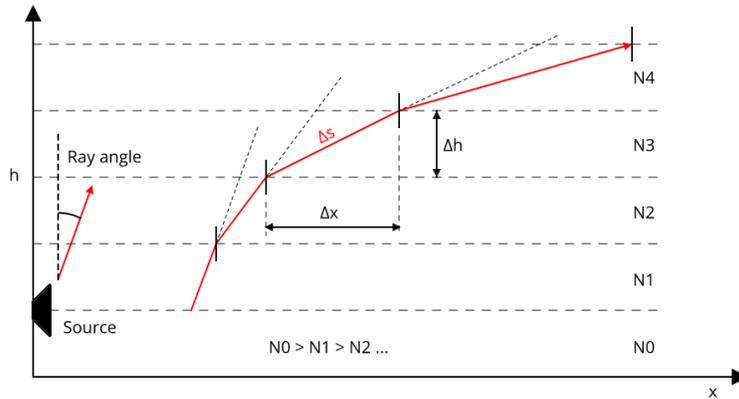
Fig. 2. The impact of the gradient of refractivity on the propagation of electromagnetic waves
