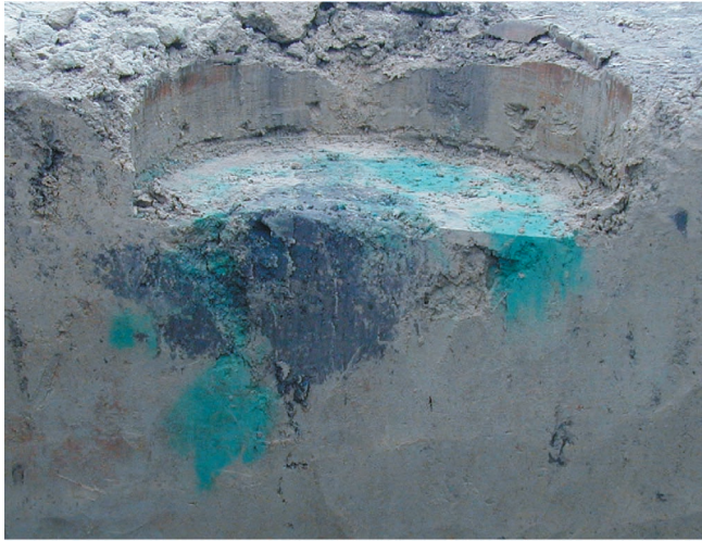
Fig. 1 The soil profile below excavated infiltration ring
