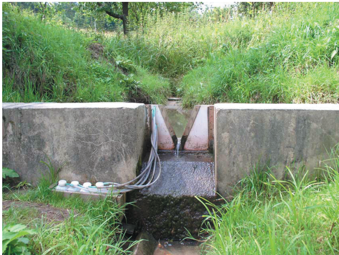
Photo 1. Water quality sampling - small Thomson weir, Rybárik basin (Pekárová, May, 2005).
