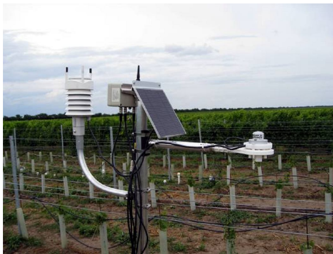
Fig. 1: Measuring station with RTU, solar panel and weather instruments (photo: R. Nolz)
