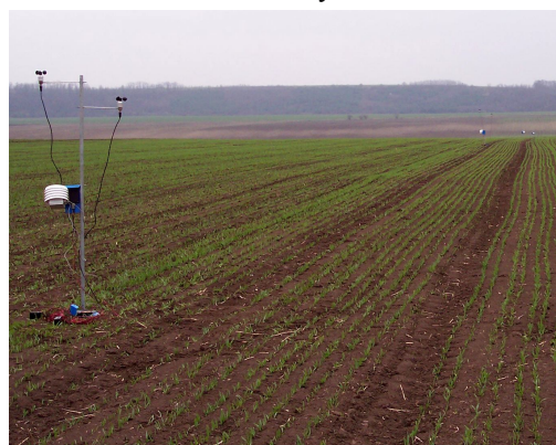
Figure 4. Measuring of horizontal profile of wind speed on leeward side of shelterbelt
