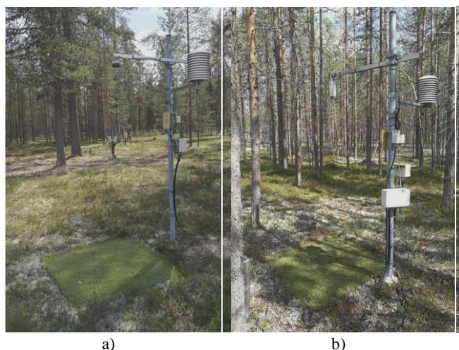
**Figure 3.** Automatic snow depth measurement with SR50 sensor a) in clearing and b) in forest at IOA. Green artificial turf is installed below the sensors.
